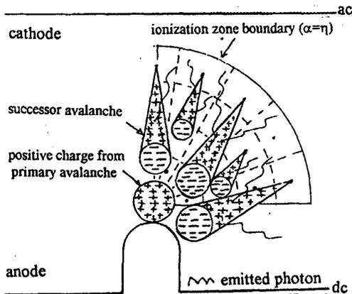
Fig.1 Growth of successor avalanches starting from the centers of sectors and ending at the positive space charge sphere or the protrusion tip.
